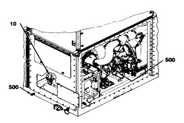
Oil Filter (Disassemble, clean housing, renew element, and reassemble.) (See note 1.) (0)
